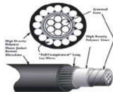
PRO-X Cable Cross Section
