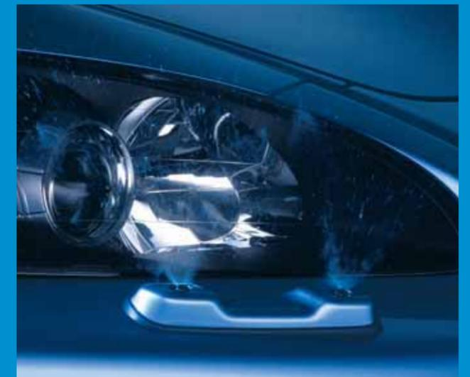
To ensure that the triple beam projector headlamps maintain their efficiency, powerful headlight washers are fitted as standard.
