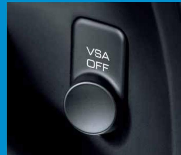
The Vehicle Stability Assist (VSA) system fitted as standard.
